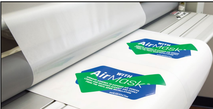
FILM BACKING: TransferRite film-based tapes are used as in a wide range of graphics applications including digital print protection, premask for air egress graphics and craft market application tape.
